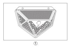
it is recommended to install vertically against the wall 2-3m high above the ground as picture @shown
